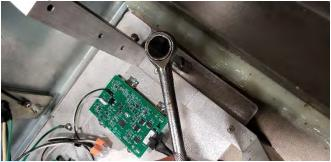
2. Adjust the cinch plate to make a tight fit to the tension plate of the fixture. Tighten the two screws on either end.
