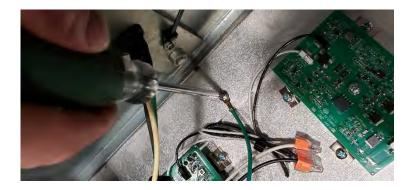
4. Connect the solid wires from the ACM plate to the incoming power wire on the power cable using wire nuts. Allow 6-pin cables to hang out of the fixture.
