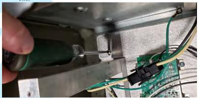
3. Attach the ground wire of the power cable to the center hole of the cinch plate using the (1) #10-32 screw and #10 lock washer in the bag provided. NOTE: Ring terminal on wire may be smaller than screw. Use force if needed to insert the screw.
