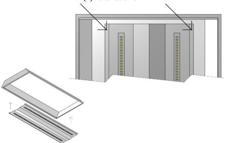
3. Reinstall lens (if applicable.) Turn on power to the luminaire.
